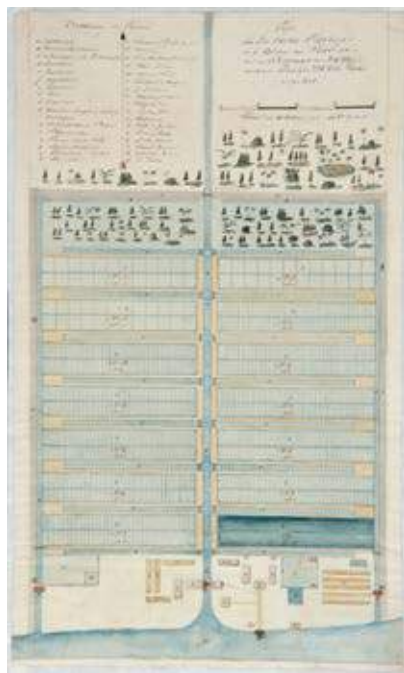
Figure 34.4 Typical drainage structure of a sugar cane plantation in Suriname (Collection Nationaal Museum van Wereldculturen. Coll.no. (source: TM-H-3350)
